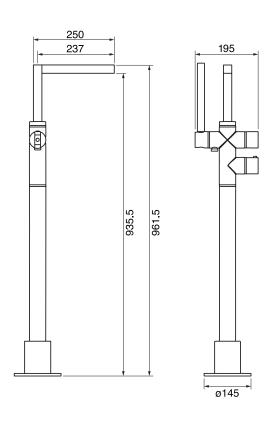
Includes rough-in 8 GPM (30.3 L/min.)
