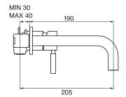
One piece rough-in Drain not included 1.5 GPM (5.7 L/min.)
