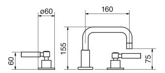
Includes push drain 1.5 GPM (5.7 L/min.)
