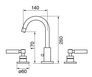
Includes push drain 1.5 GPM (5.7 L/min.)
