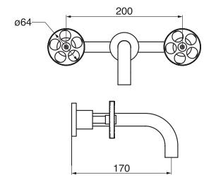
Includes one piece rough-in Drain not included 1.5 GPM (5.7 L/min.)
