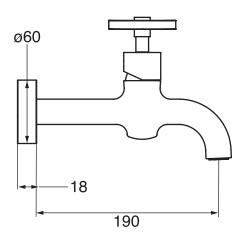
Drain not included 1.5 GPM (5.7 L/min.)
