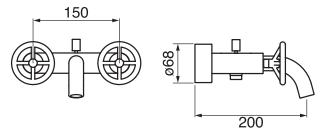
Hand shower on separate wall hook 5.3 GPM (20 L/min.)
