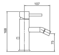
Includes mechanical pop up drain 3/8" flexible supply hoses Swivel aerator
