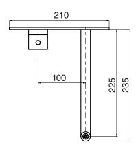
Square trim only – order rough-in separately Drain not included 2.2 GPM (8.3 L/min.)
