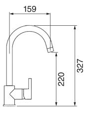
Swivel spout 1.75 GPM (6.6 L/min.)
