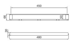
Recommend that brackets are mounted into studs
