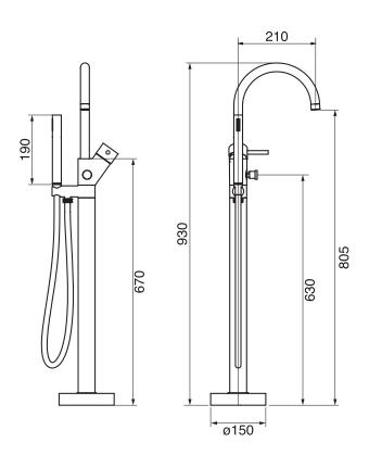
Includes rough-in 5 GPM (18.9 L/min.)
