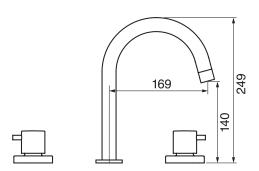
Includes push drain 1.5 GPM (5.7 L/min.)
