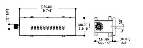
Built-in, stainless steel material Wavy rain function, with a 15° water balancing movement 2.2 GPM (8.3 L/min.) Rough not included
