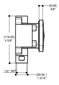
Directional head Easy clean nozzles 1.5 GPM (5.7 L/min.) Rough not included
