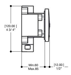
Directional head Easy clean nozzles 1.5 GPM (5.7 L/min.) Rough not included
