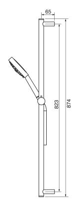
Includes bar, hose and hand shower 3 position spray Easy clean nozzles 2.5 GPM (9.5 L/min.)
