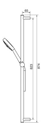
Includes bar, hose and hand shower 3 position spray Easy clean nozzles 2.5 GPM (9.5 L/min.)
