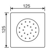
Directional head Easy clean nozzles 1.5 GPM (5.7 L/min.)
