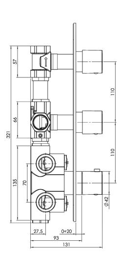
Can add independent flow control Integrated service stops, filters & back-flow preventers Rough-in can be mounted horizontally or vertically 13 GPM (49.2 L/min.)
