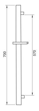
Includes bar, hose and hand shower 3 position spray with massage Easy clean nozzles 2.5 GPM (9.5 L/min.)
