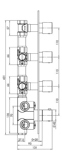
Can add independent flow control Integrated service stops, filters & back-flow preventers 13 GPM (49.2 L/min.)
