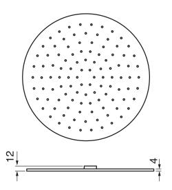
4 mm in thickness Easy clean nozzles High polished stainless steel 2.5 GPM (9.5 L/min.)
