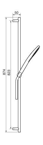
Includes bar, hose and hand shower 2 position spray Easy clean nozzles 2.5 GPM (9.5 L/min.)
