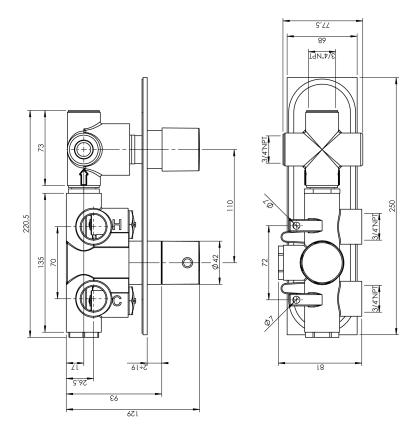
Can add independent flow control Integrated service stops, filters & back-flow preventers Rough-in can be mounted horizontally or vertically 12 GPM (45.4 L/min.)
