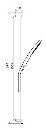
Includes bar, hose and hand shower 2 position spray Easy clean nozzles 2.5 GPM (9.5 L/min.)
