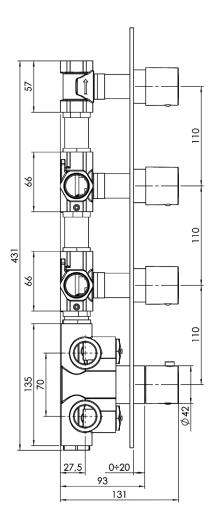
Can add independent flow control Integrated service stops, filters & back-flow preventers 13 GPM (49.2 L/min.)
