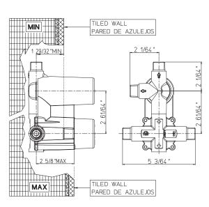
Integrated service stops, filters & back-flow preventers Easy control handle with temperature & flow control Can support two shower functions 5.6 GPM (21.2 L/min.) Extension kit available
