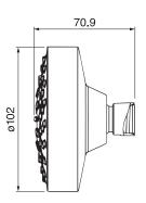
Large diameter face – 4" Easy clean nozzles 3 position spray with massage 2.2 GPM (8.3 L/min.)
