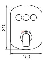
Thermostatic valve with PushGo technology – 3 controls Multiple outlets can be run simultaneously Includes rough-in Instant flow when on 5 GPM (18.9 L/min.)
