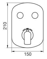
Thermostatic valve with PushGo technology – 2 controls Multiple outlets can be run simultaneously Includes rough-in Instant flow when on 5 GPM (18.9 L/min.)
