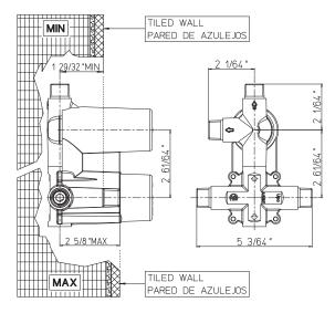
Integrated service stops, filters & back-flow preventers Easy control handle with temperature & flow control Can support two shower functions 5.6 GPM (21.2 L/min.) Extension kit available
