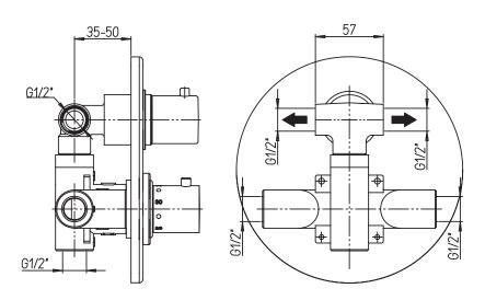
Operates one function at a time 5.6 GPM (21.2 L/min.) Extension kit available
