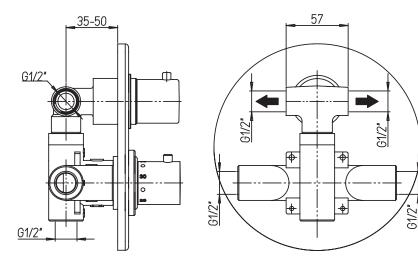
Operates one function at a time 5.6 GPM (21.2 L/min.) Extension kit available
