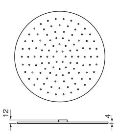
4 mm in thickness Easy clean nozzles High polished stainless steel 2.5 GPM (9.5 L/min.)
