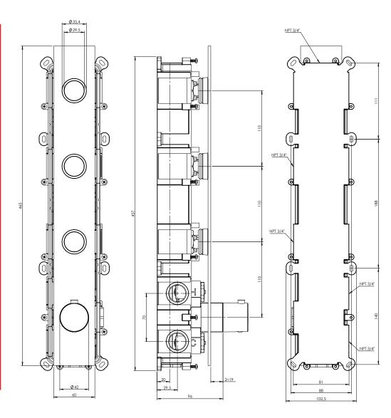
Can add independent control Integrated service stops, filters & back-flow preventers 100% flow when on 13 GPM (49.2 L/min.) Extension available
