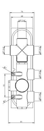
Can add independent flow control Integrated service stops, filters & back-flow preventers 12 GPM (45.4 L/min.)
