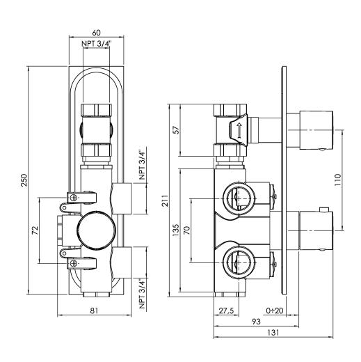
Can add independent flow control Integrated service stops, filters & back-flow preventers Rough-in can be mounted horizontally or vertically 10 GPM (37.8 L/min.)
