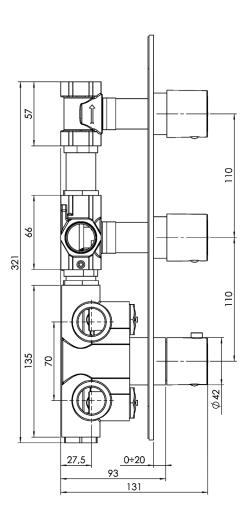
Can add independent flow control Integrated service stops, filters & back-flow preventers Rough-in can be mounted horizontally or vertically 13 GPM (49.2 L/min.)
